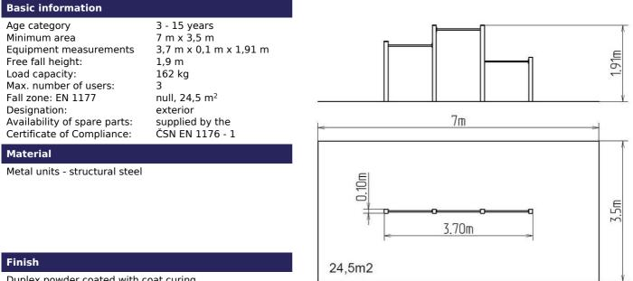
Duplex powder coated with coat curing Hot-dip galvanizing
