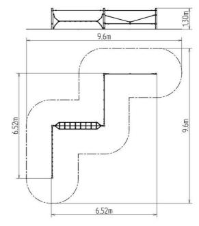
The support structures of the rope unit are made from structural steel, they are zinc coated or duplex powder coated with coat curing according to RAL to prevent corrosion and fixed in a concrete bed. The ropes are made using HERKULES material (16 mm thick ropes made from polypropylene with a steel internal core) and are connected with plastic joints. All fastening material is galvanized or stainless steel.
