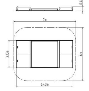
The sandbox is made of glued prisms. This solution provides maximum protection against cracks that are common in off-wood wood products. The surface treatment of these prisms consists in the impregnation and three-layer application of the top glazing varnish, which meets the requirements of EN 71/3 (safe for children's toys).
