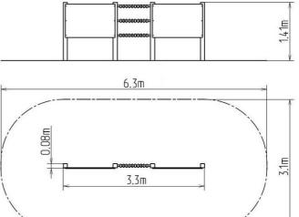
Metal parts - structural steel Wooden parts - water-proof plywood
