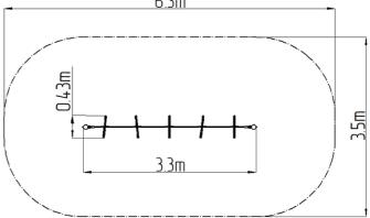
The support structures of the rope unit are made from structural steel, they are zinc coated or duplex powder coated with coat curing according to RAL to prevent corrosion and fixed in a concrete bed. The ropes are made using HERKULES material (16 mm thick ropes made from polypropylene with a steel internal core) and are connected with plastic joints. All fastening material is galvanized or stainless steel.
