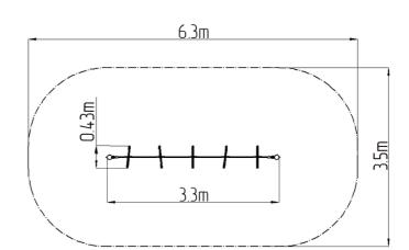
The support structures of the rope unit are made from structural steel, they are zinc coated or duplex powder coated with coat curing according to RAL to prevent corrosion and fixed in a concrete bed. The ropes are made using HERKULES material (16 mm thick ropes made from polypropylene with a steel internal core) and are connected with plastic joints. All fastening material is galvanized or stainless steel.
