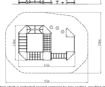
The support structure of the skill path is made of structural steel which is protected against corrosion by zinc coating, resulting in a very prolonged service life of the workout elements or duplex powder coated with coat curing according to RAL to prevent corrosion. These structures are embedded in a concrete base. All other metallic elements are also zinc coated or duplex powder coated with coat curing according to RAL to prevent corrosion.
