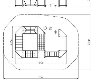
The support structure of the skill path is made of structural steel which is protected against corrosion by zinc coating, resulting in a very prolonged service life of the workout elements or duplex powder coated with coat curing according to RAL to prevent corrosion. These structures are embedded in a concrete base. All other metallic elements are also zinc coated or duplex powder coated with coat curing according to RAL to prevent corrosion.
