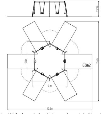
The support structure of the swing is made from structural steel, which is zinc coated or duplex powder coated with coat curing according to RAL to prevent corrosion. The structures are anchored into the ground in steel plates, which are protected against corrosion by hot-dip galvanizing a and fixed in a concrete bed. The anchors are fastened to the play unit with bolts and their structure ensures that they are not in direct contact with the ground.
