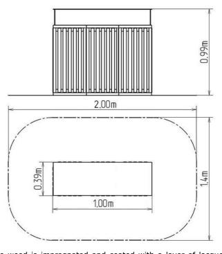
The waste bin for sorted waste is made from spruce wood. The wood is impregnated and coated with a layer of lacquer. The structure is fixed in a concrete bed. The metal frame and the insert of the litter bin are made from galvanized steel. All metal units are protected against corrosion by hot-dip galvanizing. All fastening material is galvanized or stainless steel. Cubic capacity: 3x60 l
