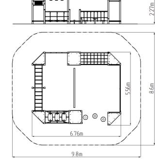
The support structure of the skill path is made of structural steel which is protected against corrosion by zinc coating, resulting in a very prolonged service life of the workout elements or duplex powder coated with coat curing according to RAL to prevent corrosion. These structures are embedded in a concrete base. All other metallic elements are also zinc coated or duplex powder coated with coat curing according to RAL to prevent corrosion.
