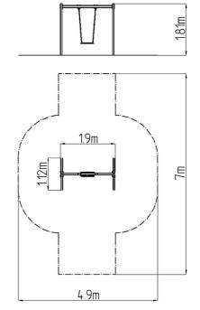
The support structure of the swing is made from structural steel, which is zinc coated or duplex powder coated with coat curing according to RAL to prevent corrosion and is fixed in a concrete bed. The Normal seat is made of aluminum, covered with a soft and comfortable rubber. The chains are stainless steel, resulting in a very prolonged service life of the product. All fastening material is galvanized or stainless steel.
