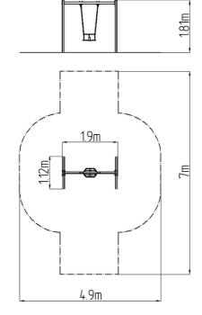
The support structure of the swing is made from structural steel, which is zinc coated and KOMAXIT powder coated according to the RAL colour chart and is fixed in a concrete bed. The Normal seat is made of aluminum, covered with a soft and comfortable rubber.
