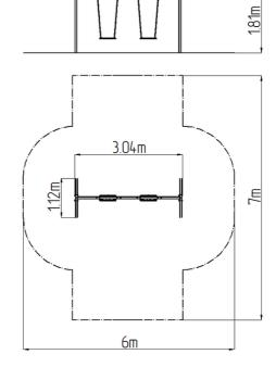
The support structure of the swing is made from structural steel, which is zinc coated or duplex powder coated with coat curing according to RAL to prevent corrosion and is fixed in a concrete bed. The Normal seat is made of aluminum, covered with a soft and comfortable rubber. The chains are stainless steel, resulting in a very prolonged service life of the product. All fastening material is galvanized or stainless steel.
