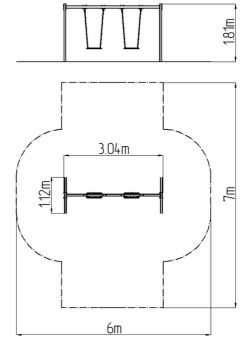
The support structure of the swing is made from structural steel, which is zinc coated and KOMAXIT powder coated according to the RAL colour chart and is fixed in a concrete bed. The Normal seat is made of aluminum, covered with a soft and comfortable rubber. The chains are stainless steel, resulting in a very prolonged service life of the product. All fastening material is galvanized or stainless steel.
