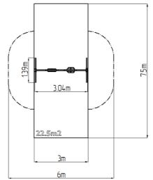
The support structure of the swing is made from structural steel, which is zinc coated and KOMAXIT powder coated according to the RAL colour chart and is fixed in a concrete bed. The Baby seat is made of rubber and is reinforced with an aluminum insert. The Normal seat is made of aluminum, covered with a soft and comfortable rubber. The chains are stainless steel, resulting in a very prolonged service life of the product. All fastening material is galvanized or stainless steel.
