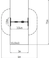
The support structure of the swing is made from structural steel, which is zinc coated and KOMAXIT powder coated according to the RAL colour chart and is fixed in a concrete bed. The Baby seat is made of rubber and is reinforced with an aluminum insert. The Normal seat is made of aluminum, covered with a soft and comfortable rubber. The chains are stainless steel, resulting in a very prolonged service life of the product. All fastening material is galvanized or stainless steel.
