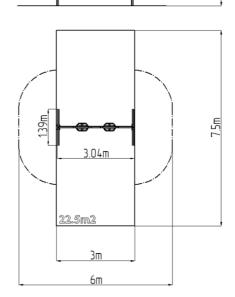
The support structure of the swing is made from structural steel, which is zinc coated or duplex powder coated with coat curing according to RAL to prevent corrosion and is fixed in a concrete bed. The Baby seat is made of rubber and is reinforced with an aluminum insert. The chains are stainless steel, resulting in a very prolonged service life of the product. All fastening material is galvanized or stainless steel.
