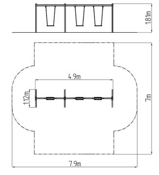
The support structure of the swing is made from structural steel, which is zinc coated or duplex powder coated with coat curing according to RAL to prevent corrosion and is fixed in a concrete bed. The Normal seat is made of aluminum, covered with a soft and comfortable rubber. The chains are stainless steel, resulting in a very prolonged service life of the product. All fastening material is galvanized or stainless steel.
