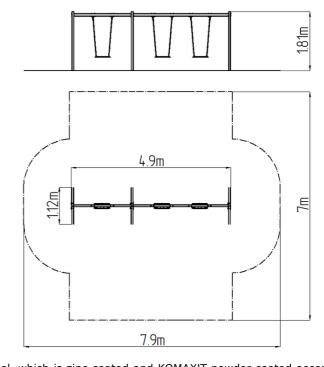
The support structure of the swing is made from structural steel, which is zinc coated and KOMAXIT powder coated according to the RAL colour chart and is fixed in a concrete bed. The Normal seat is made of aluminum, covered with a soft and comfortable rubber. The chains are stainless steel, resulting in a very prolonged service life of the product. All fastening material is galvanized or stainless steel.
