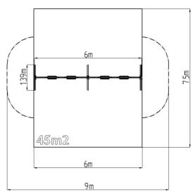
The support structure of the swing is made from structural steel, which is zinc coated and KOMAXIT powder coated according to the RAL colour chart and is fixed in a concrete bed. The Normal seat is made of aluminum, covered with a soft and comfortable rubber. The chains are stainless steel, resulting in a very prolonged service life of the product. All fastening material is galvanized or stainless steel.
