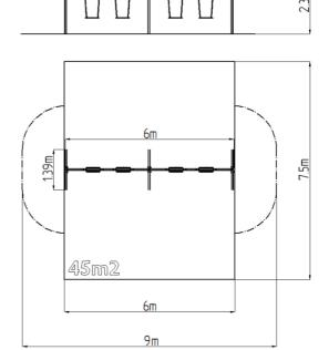
The support structure of the swing is made from structural steel, which is zinc coated or duplex powder coated with coat curing according to RAL to prevent corrosion and is fixed in a concrete bed. The Normal seat is made of aluminum, covered with a soft and comfortable rubber. The chains are stainless steel, resulting in a very prolonged service life of the product. All fastening material is galvanized or stainless steel.
