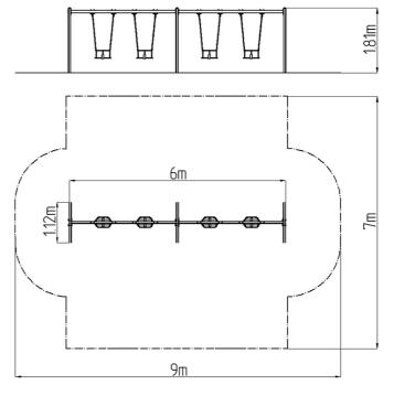
The support structure of the swing is made from structural steel, which is zinc coated and KOMAXIT powder coated according to the RAL colour chart and is fixed in a concrete bed. The Baby seat is made of rubber and is reinforced with an aluminum insert. The chains are stainless steel, resulting in a very prolonged service life of the product. All fastening material is galvanized or stainless steel.
