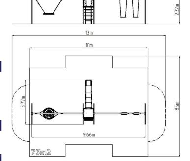
The load-bearing structure of the double-shaft is made of structural steel, which is protected against corrosion by zinc coating, which results in a very significant extension of the life of the play element or duplex powder coated with coat curing according to RAL to prevent corrosion. These structures are embedded in a concrete bed. All other metallic elements are also zinc coated or duplex powder coated with coat curing according to RAL to prevent corrosion.
