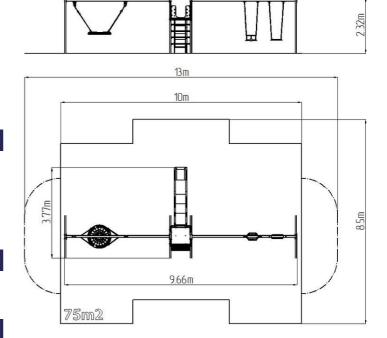
The load-bearing structure of the double-shaft is made of structural steel, which is protected against corrosion by zinc coating, which results in a very significant extension of the life of the play element and fired paint KOMAXIT according to RAL. These structures are embedded in a concrete bed. All other metal elements are also treated with galvanizing and fired with KOMAXIT RAL.
