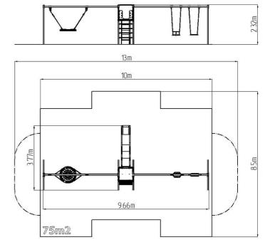
The load-bearing structure of the double-shaft is made of structural steel, which is protected against corrosion by zinc coating, which results in a very significant extension of the life of the play element and fired paint KOMAXIT according to RAL. These structures are embedded in a concrete bed. All other metal elements are also treated with galvanizing and fired with KOMAXIT RAI.
