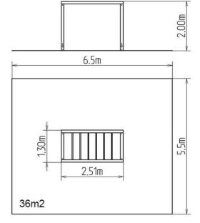
The support structure of the climbing set is made from structural steel (steel profile 100 x 100 mm), it is zinc coated which significantly prolongs the life of the play unit and KOMAXIT powder coated according to the RAL colour chart and it is fixed in a concrete bed. All other metal units are zinc coated and KOMAXIT powder coated according to the RAL.
