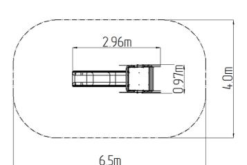
The support structure of the slide is made from structural steel, which is zinc coated or duplex powder coated with coat curing according to RAL to prevent corrosion and is fixed in a concrete bed. All metal units are zinc coated or duplex powder coated with coat curing according to RAL to prevent corrosion.
