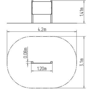
The support structure of the drawing board is made of structural steel which is protected against corrosion by zinc coating, resulting in a very prolonged service life of the workout elements or duplex powder coated with coat curing according to RAL to prevent corrosion. These structures are anchored to concrete footings. All other metallic elements are also zinc coated or duplex powder coated with coat curing according to RAL to prevent corrosion.
