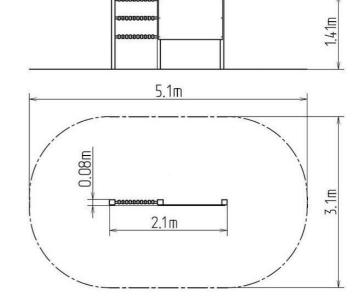
The support structure of the drawing board is made of structural steel which is protected against corrosion by zinc coating, resulting in a very prolonged service life of the workout elements or duplex powder coated with coat curing according to RAL to prevent corrosion. These structures are anchored to concrete footings. All other metallic elements are also zinc coated or duplex powder coated with coat curing according to RAL to prevent corrosion.
