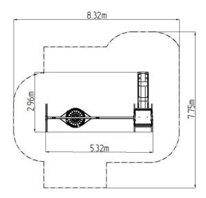
Metal parts - structural steel Slide - fibreglass Plastic parts - HDPE Platform - HPL Suspension ropes NEST - polypropylene with inner steel core Rope seat NEST - high-strength fiber polypropylene
