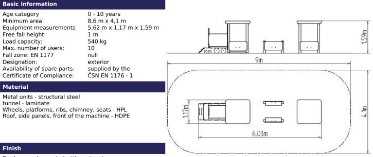
Duplex powder coated with coat curing Hot-dip galvanizing
