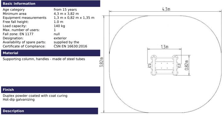
The handles are made of powder-coated steel tubes. The supporting column is made of a steel tube with a mounting flange at the bottom. The frame and tread are made of powder coated sheet metal. Rolling bearings are used for movable connections. Holes are sealed with steel elements at the ends. All fasteners are stainless.
