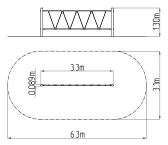
The support structures of the rope unit are made from structural steel, they are zinc coated or duplex powder coated with coat curing according to RAL to prevent corrosion and fixed in a concrete bed. The ropes are made using HERKULES material (16 mm thick ropes made from polypropylene with a steel internal core) and are connected with plastic joints. All fastening material is galvanized or stainless steel.
