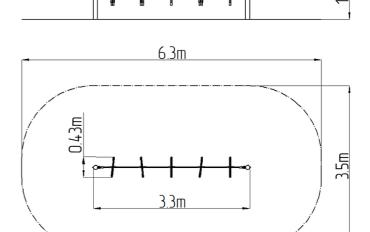
The support structures of the rope unit are made from structural steel, they are zinc coated or duplex powder coated with coat curing according to RAL to prevent corrosion and fixed in a concrete bed. The ropes are made using HERKULES material (16 mm thick ropes made from polypropylene with a steel internal core) and are connected with plastic joints. All fastening material is galvanized or stainless steel.
