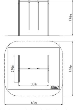
The support structure of the climbing set is made from structural steel, it is zinc coated which significantly prolongs the life of the play unit or duplex powder coated with coat curing according to RAL to prevent corrosion and it is fixed in a concrete bed. All other metal units are zinc coated or duplex powder coated with coat curing according to RAL to prevent corrosion. Climbing rope is made of jute (diameter 35mm). All fastening material is galvanized or stainless steel.
