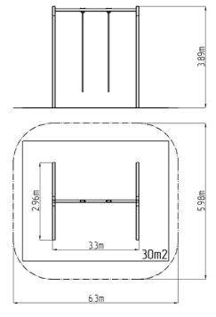
The support structure of the climbing set is made from structural steel, it is zinc coated which significantly prolongs the life of the play unit or duplex powder coated with coat curing according to RAL to prevent corrosion and it is fixed in a concrete bed. All other metal units are zinc coated or duplex powder coated with coat curing according to RAL to prevent corrosion. Climbing rope is made of jute (diameter 35mm). All fastening material is galvanized or stainless steel.
