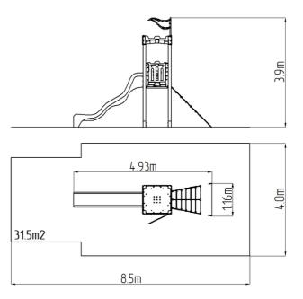
The support structure of the tower unit is made of structural steel which is protected against corrosion by zinc coating, resulting in a very prolonged service life or duplex powder coated with coat curing according to RAL to prevent corrosion. All other metallic elements are also zinc coated or duplex powder coated with coat curing according to RAL to prevent corrosion.
