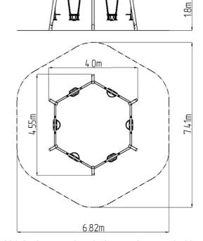
The support structure of the swing is made from structural steel, which is zinc coated or duplex powder coated with coat curing according to RAL to prevent corrosion. The structures are anchored into the ground in steel plates, which are protected against corrosion by hot-dip galvanizing a and fixed in a concrete bed. The anchors are fastened to the play unit with bolts and their structure ensures that they are not in direct contact with the ground.
